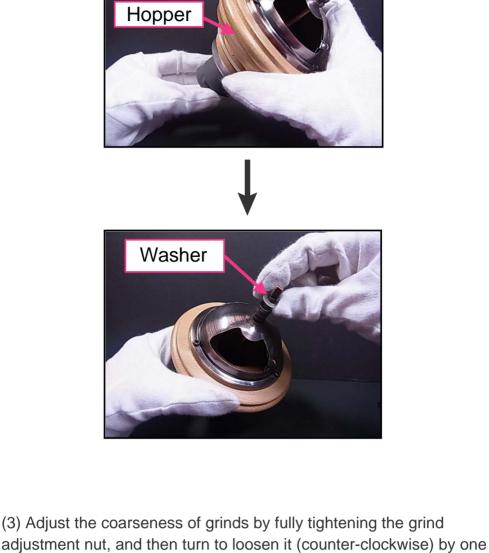
forwards, align the indent of the grind adjustment nut with the cut section, then rotate one notch at a time to adjust the grind by the number of notches rotated.
